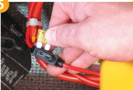
Replace the 20 amp fuse to the inline fuse holder on the positive side of the 130 amp hour battery.
