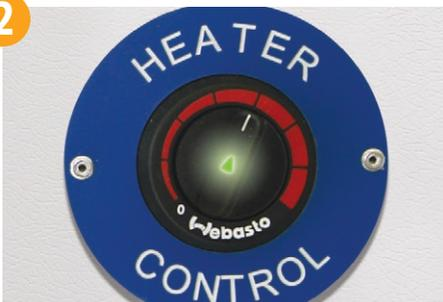
Turn the heater control clockwise to the "on" position, so that the error code is being given.
